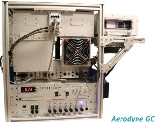
equipped with two-stage thermal desorption preconcentration system
